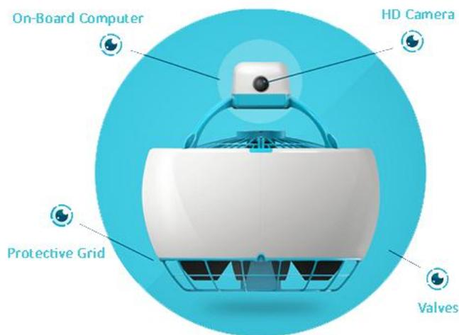
**Fig. 1 Design of ORBOT**
