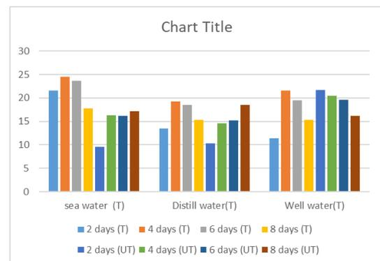
Figure 3: (b). Tensile strength of 10 mm palm composite.
